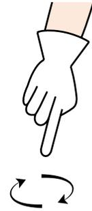
**Unwind:** With arm extended downward and forefinger pointing down, move hand in small horizontal circles.
