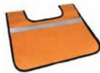
Wire Rope Dampener: Reduces risk of injury due to recoil in event of a winch line or recovery strap failure (whip effect). Shape of blanket with pockets can be filled with weights like sand or stones. Once loaded should be folded around wire rope before pulling.
